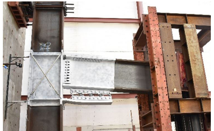
Fig. 4. DFF Arrow connection at 6% drift (Lee and Uang 2021)
