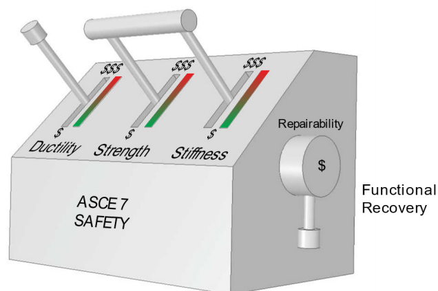
Fig. 7 The repairability lever is a way to control functional recovery
