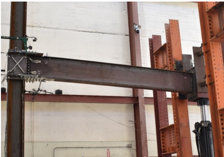
Fig. 4 Experimental Test Without Lateral Bracing (W21X50 shown)
